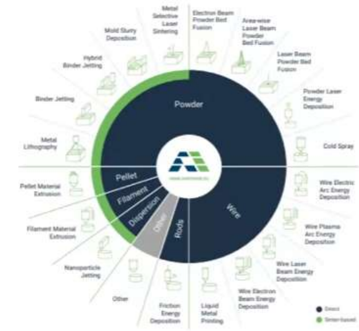
FIGURE 15 METAL ADDITIVE MANUFACTURING TECHNOLOGY MAP
